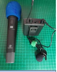
Use either the handheld mic' or the bodypack with tie mic' or headset mic' plugged in to it
